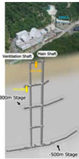
Fig.2 Cross section of MIU(500m depth), and location s of STG100 & STG200 borehole site (φ 98mm, 20m depth). Modified from JAEA report; http://www.jaea.go.jp/04/tono/miu_e/weeklyweekliumiu.html .
