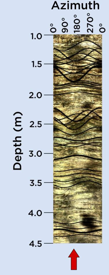
+ We drilled seven boreholes and counted fractures in each Optical hole with an Televiewer.
