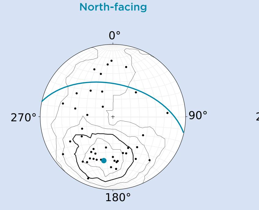
+ Fractures on the north- and south-facing slope trend in the same direction. Points represent poles to planes of fractures; dark contours identify significant fracture orientations; colored arcs and points represent mean strike and dip of significant fractures.
