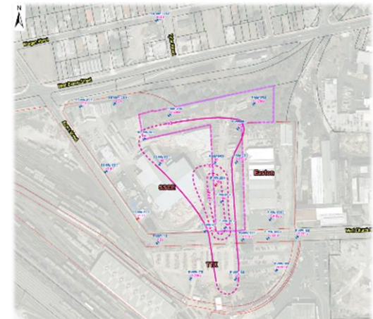
Shallow Sand Unit Naphthalene Isoconcentration Map
