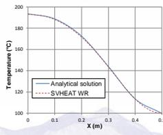
Temperature versus position (x = y) at 0.25 days.
