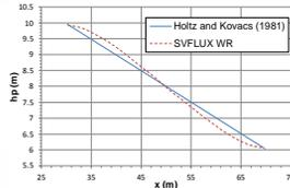
The contour of head (h) and select streamlines under the dam
