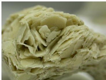
Calcium Sulfate Scale from a Column Pipe
