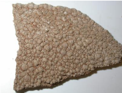
Calcium Carbonate Scale from a Well
