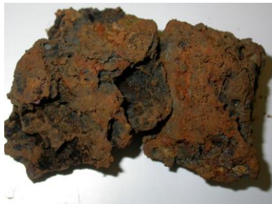
Iron Oxide Scale from a Well
