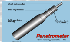
Unconfined Compressive Strength
